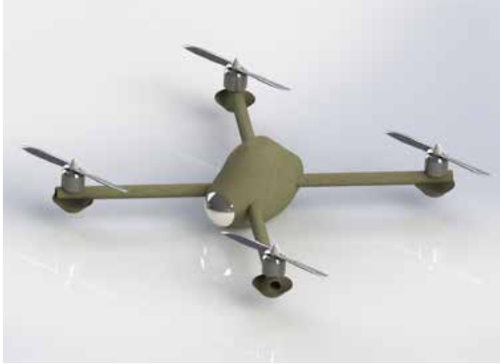
Phoenix drone concept (indoor version, collision avoidance system and propeller protection not shown). Composite materials that can sustain up to 1000 °C. Internal cooling and heat shields for external components would be used. The motor-to-motor span is under 50 cm.
